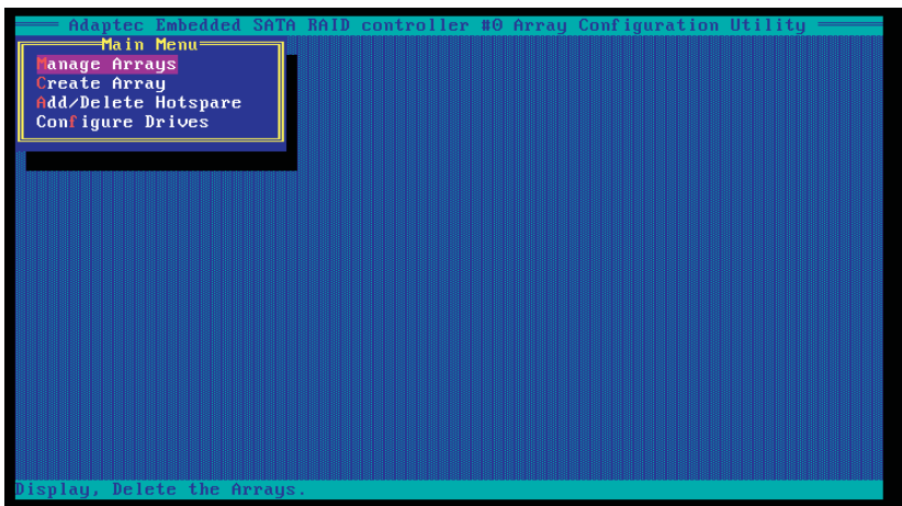
Figure 2-5. Adaptec RAID Utility Program Screen
