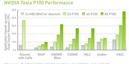
CPU: 16 cores, E5-2698v3 @ 2.30GHz. 256GB System Memory. Tesla K80 GPUs: 2x Dual GPU K80s, Pre-Production Tesla P100
