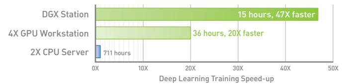
DGX Station performance projected based on DGX-1 (with Tesla V100) Workload: ResNet50, 90 epochs to solution | CPU Server: Dual Xeon E5-2699 v4, 2.6GHz. Projections subject to change.
