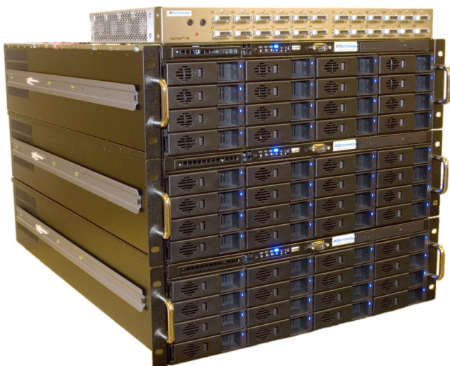
48 TB, 3 Server ServaStor IB Storage Cluster - Can be added to an existing data center's standard 19" rack
