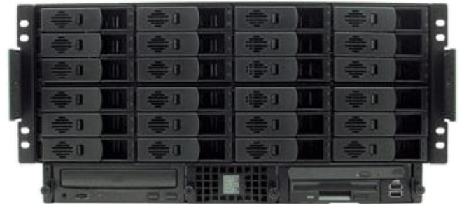
Microway 5U NAS Server with 18 TB raw storage
