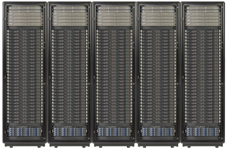
4320-core HPC Cluster with 56 Gbit/sec FDR InfiniBand
