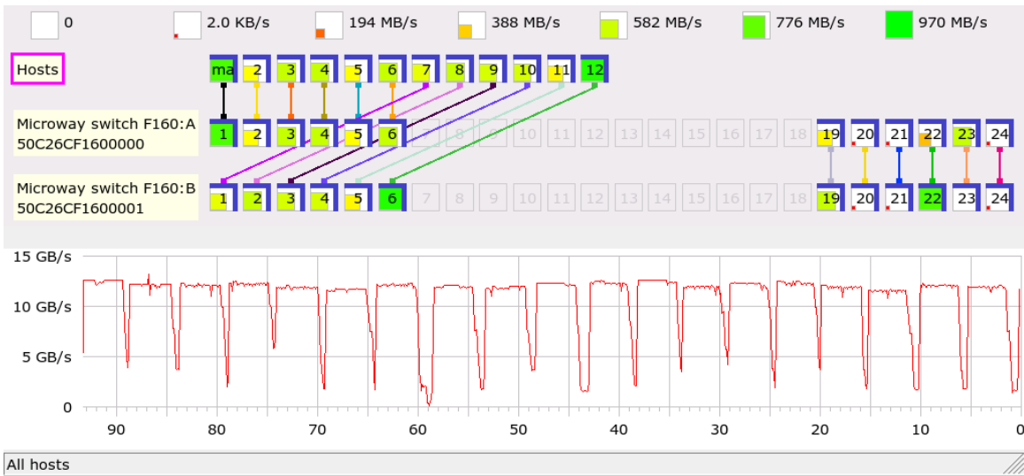
Figure 20: Case study with 6 interswitch cables.
