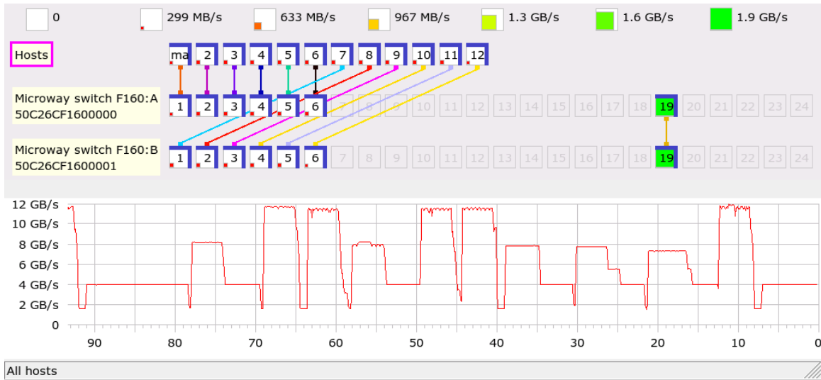
Figure 16: Case study to determine how much bandwidth is needed between two switches. flop is running, and there is one cable between switch F160:A and F160:B.
