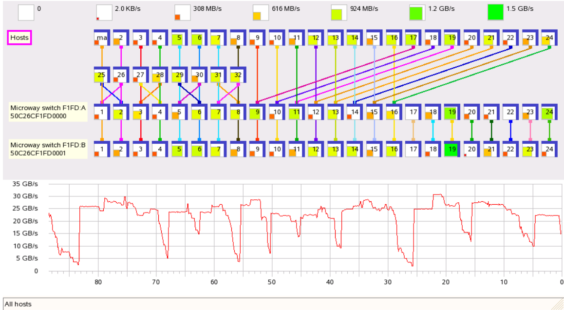
Figure 8: Two instances of flop are running at the same time, leading to a highly irregular traffic pattern.
