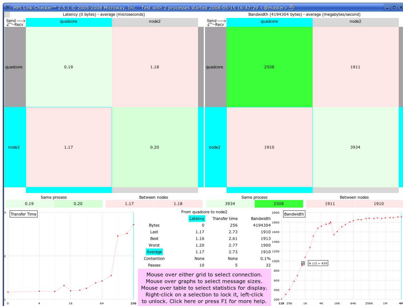
Figure 2: MPI Link-Checker shows latency below 1.2 microseconds in TriCom-X HCAs using PCI Express Gen 2.
