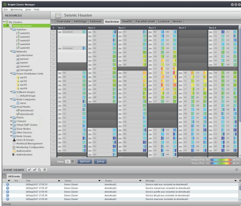
The status of cluster nodes, switches, other hardware, as well as up to six metrics can be visualized in the Rackview. A zoom-out option is available for clusters with many racks.
