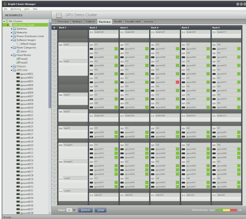
Cluster health checks can be visualized in the Rackview. This screenshot shows that GPU unit 41 fails a health check called "AllFansRunning".
